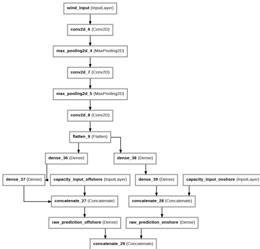
Figure 3 Architecture of CNN model
